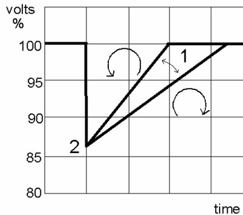
1) Adjustable slope      2) Instant of load application
